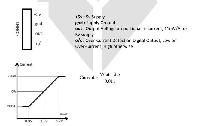
Over Current can be detected by adjusting the preset for desired value of current. Turn preset clockwise to increase current range and anti-clockwise to decrease current range. On over current, o/c pin goes low and red LED glows. Over Current cannot be set for negative values of current
