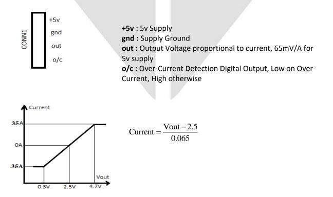
Over Current can be detected by adjusting the preset for desired value of current. Turn preset clockwise to increase current range and anti-clockwise to decrease current range. On over current, o/c pin goes low and red LED glows. Over Current cannot be set for negative values of current
