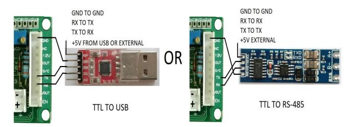
**MODBUS:** The device can be configures as a Modbus slave. Default Slave ID is 1. To change this value, send character 'I' through the Serial Port. Following message will be displayed "Enter new Slave ID". Type the new value and press Enter. Restart the system. Only valid slave IDs from 1 to 247 are permitted.
