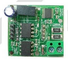
**Description:** VVM101 Digital Voltage Sensor Module provides economical and precise isolated DC voltage measurement solution for industrial and commercial applications. It allows system designers to safely monitor line voltage. Measured voltage is digitally available on Serial UART TTL interface. This interface can also be connected to RS232/RS485 systems
