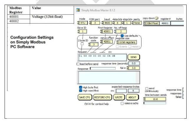
In Modbus slave Mode, regular Serial UART communication will not be available, because the data will be communicated via Modbus protocol. To exit Modbus slave mode, send **SERIALON** message via the Serial Port. "Serial Mode Selected" message appears and device restarts into regular Serial mode.
