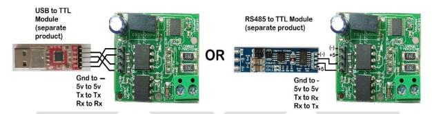
**MODBUS:** The device can be configured as a Modbus slave. Default Slave ID is 1. To change this value, send command **SLVXXX** through the Serial Port, where XXX denotes Slave ID from 001 to 247. Only valid slave IDs from 001 to 247 are permitted. For example to set Slave ID as 5, send **SLV005.** To enter Modbus slave mode, send **MOD** through the Serial Port. "Modbus Mode Selected" message appears and device restarts into Modbus Mode. Register format is as follows:
