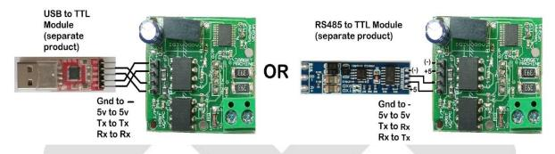
**MODBUS:** The device can be configured as a Modbus slave. Default Slave ID is 1. To change this value, send command **SLVXXX** through the Serial Port, where XXX denotes Slave ID from 001 to 247. Only valid slave IDs from 001 to 247 are permitted. For example to set Slave ID as 5, send **SLV005.** To enter Modbus slave mode, send **MOD** through the Serial Port. "Modbus Mode Selected" message appears and device restarts into Modbus Mode. Register format is as follows:
