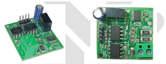
**Description:** VVM102 Digital Voltage Sensor Module provides economical and precise isolated DC voltage measurement solution for industrial and commercial applications. It allows system designers to safely monitor line voltage. Measured voltage is digitally available on Serial UART TTL interface. This interface can also be connected to RS232/RS485 systems
