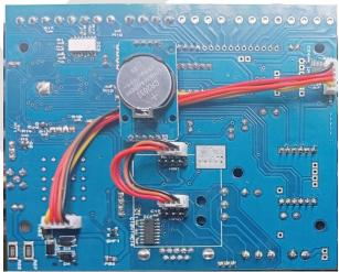
On boards without isolation, the communication section is part of the main board. For isolation, users can disconnect the short 4 pin wires and use our VVM481 TTL UART Isolator.
