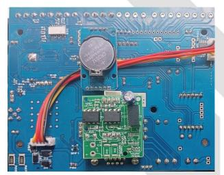
On boards provided with isolation, the RS485/RS232 communication section is optically isolated from the remaining section. Isolation: 1.5kV
