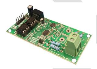
**Description:** VVM111 Digital Voltage Sensor Module provides economical and precise isolated DC voltage measurement solution for industrial and commercial applications. It allows system designers to safely monitor line voltage. Measured voltage is digitally available on Serial UART TTL interface. This interface can also be connected to RS232/RS485 systems
