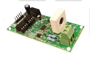
**Description:** VVM311 Digital Voltage Current Sensor Module provides economical and precise isolated DC voltage and current measurement solution for industrial and commercial applications. It allows system designers to safely monitor line voltage and current. Measured voltage is digitally available on Serial UART TTL interface. This interface can also be connected to RS232/RS485 systems
