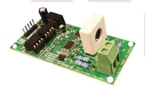
**Description:** VVM312 Digital Voltage Current Sensor Module provides economical and precise isolated DC voltage and current measurement solution for industrial and commercial applications. It allows system designers to safely monitor line voltage and current. Measured voltage is digitally available on Serial UART TTL interface. This interface can also be connected to RS232/RS485 systems
